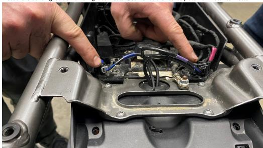
**4.** Remove the (4) 6mm screws fastening the oem license plate bracket to the subframe.
