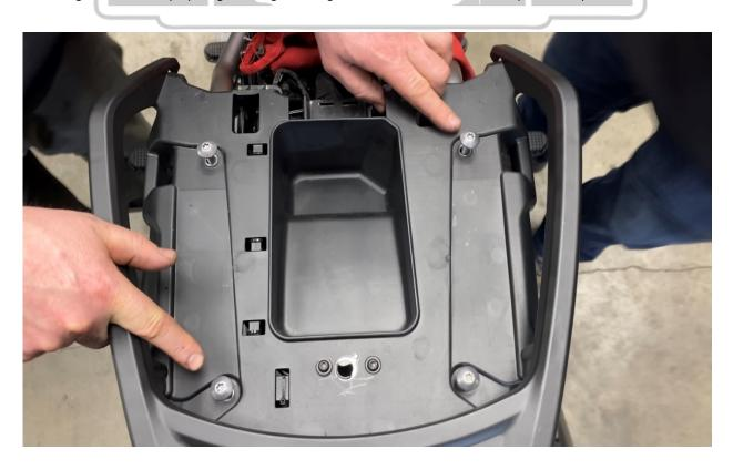
3. Disconnect the left and right side marker light connectors, as well as the license plate illuminator connector.
